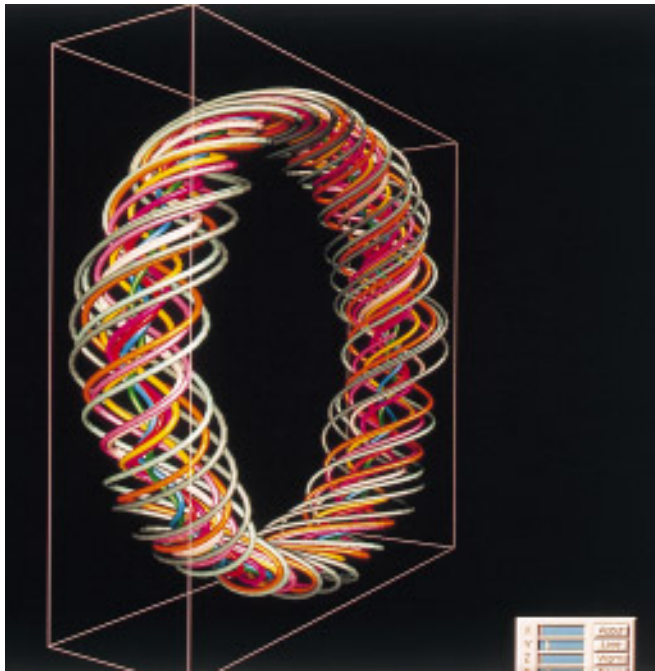
FIG. 3. A typical vortex ring with swirl. Spiral stream lines winding around stream surfaces are clearly visible. Produced in The Laboratory for Advanced Computing at The University of Illinois at Chicago by R. Grossman, J. Leigh, and A. Lifschitz.
